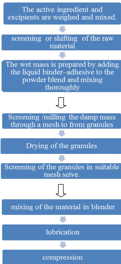
**Flowchart:- Wet granulation process.****d. Mass-Extrusion**<sup>[1,6,8]</sup>
