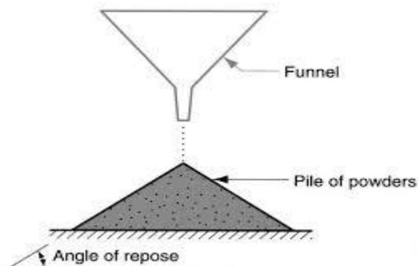
**Figure: Measurement of angle of repose (Fixed Funnel method).**
