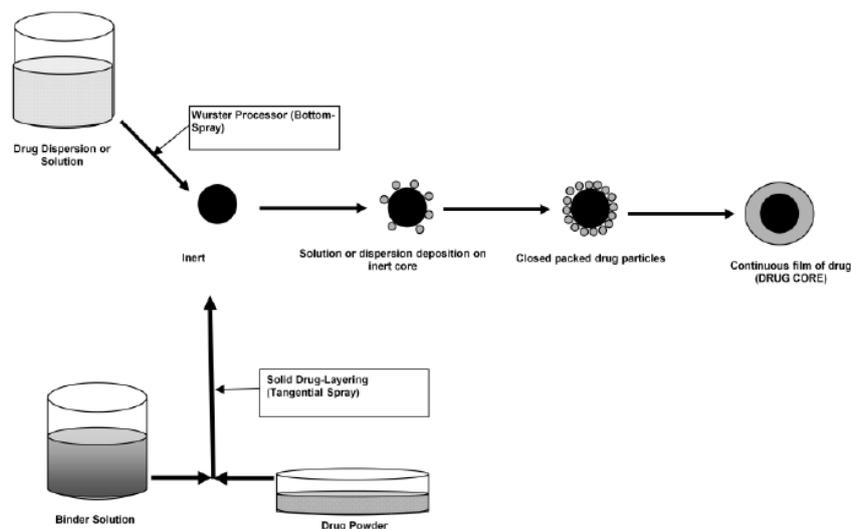
**Fig 6: Principle of Powder Layering and Solution/Suspension Layering.**
