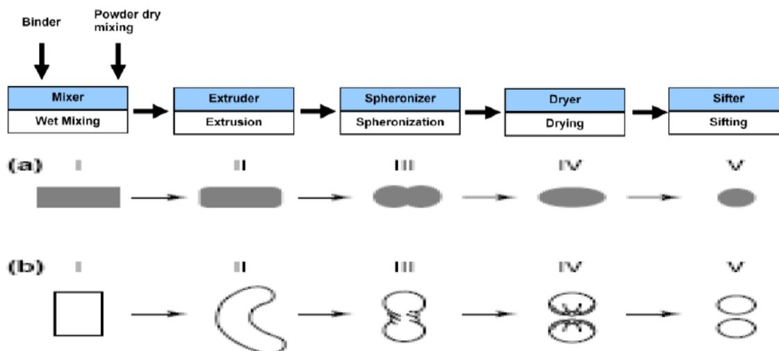
**Fig 7: Principle of Extrusion and Spheronization process.**
