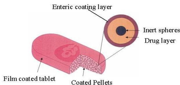
**Fig 1: MUPS - Multiple Unit Pellets compressed to Tablet.**
