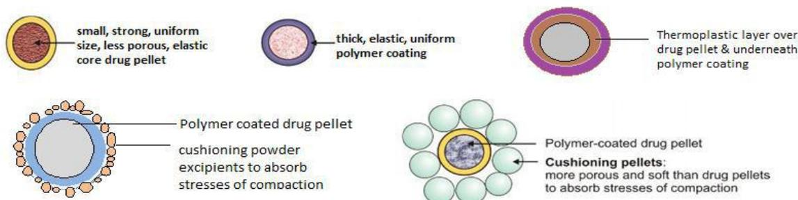
**Fig 5: Schematic representation of various approaches to prepare MUPS of coated pellet formulations.**
