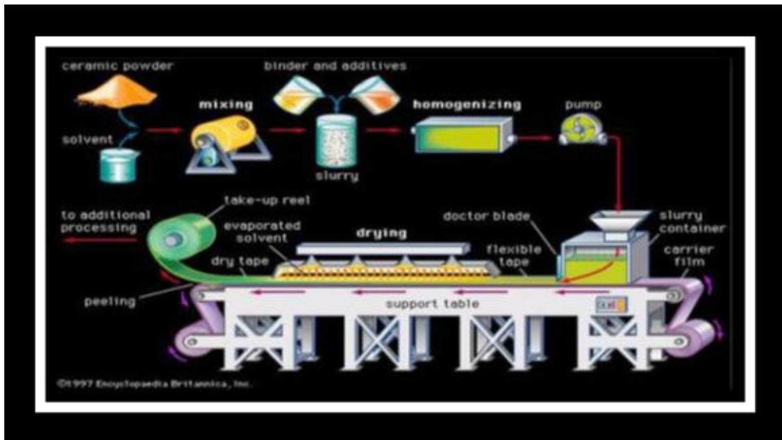
**Fig. 1: Solvent casting method.**
