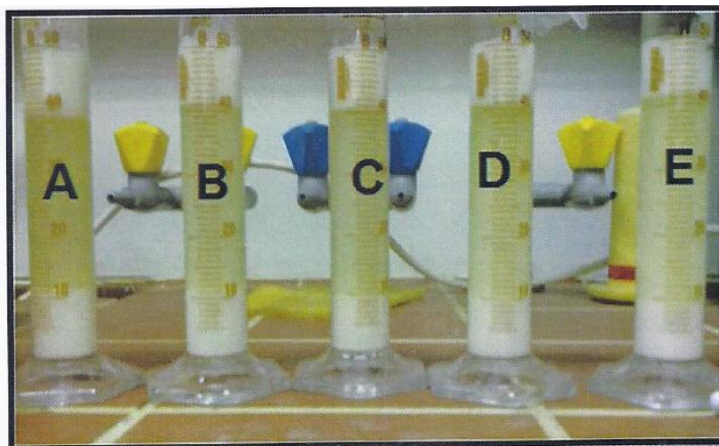
Fig. 2: sedimentation properties determination; A=25 °C, B=40 °C, C=60 °C, D=70°C, E=80 °C.
