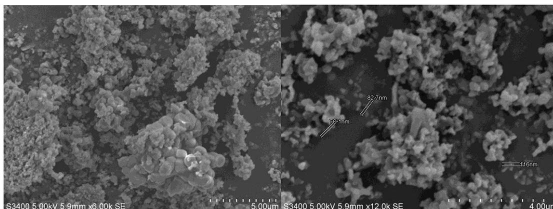
Figure 6: Surface morphology of optimized NP2 at 6000x and 12000x magnifications.
