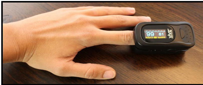
Shape: the pulse oximetry measuring the peripheral oxygen saturation.
