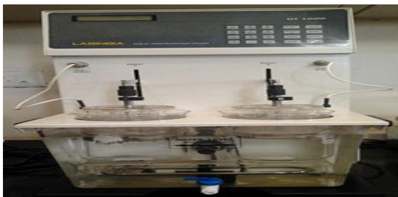
Fig. 4: In-vitro disintegration test apparatus.
