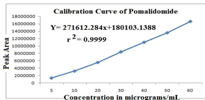
Fig. 3: Calibration curve of the Pomalidomide by RP-HPLC.
