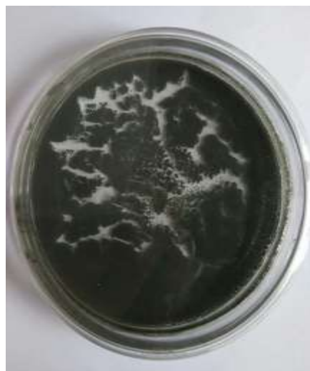
Figure 1b. Powder form of Camellia sinensis mediated iron nanoparticles
