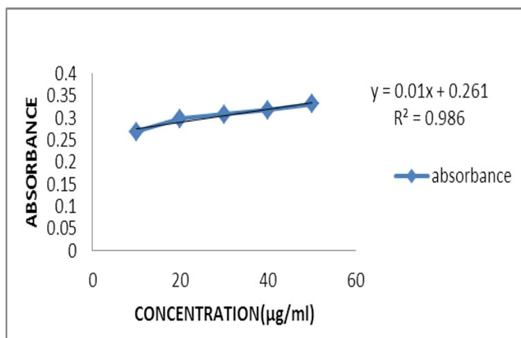
Figure 1: Calibration curve of SSD in ethanol at 241nm.
