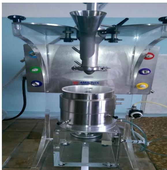
**Fig 2: Radial screw-feed extruder (4M8Trix, Procept, Belgium)**
