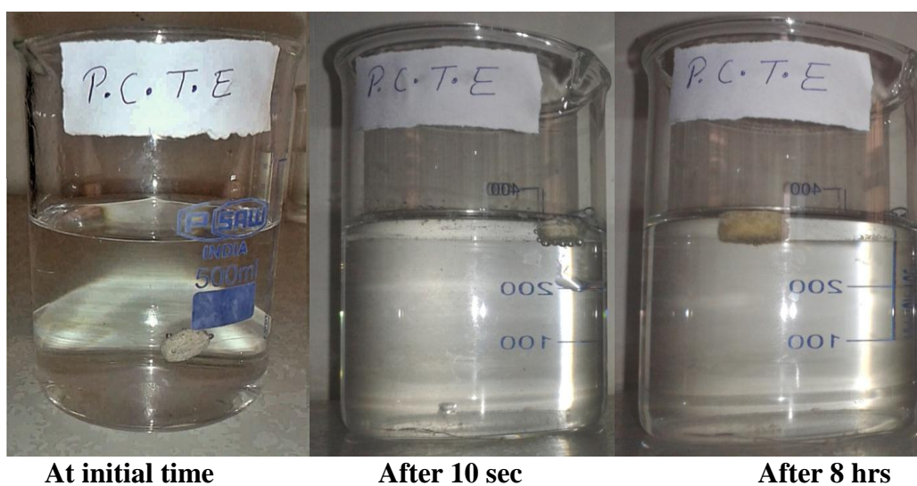
Figure no. 2: Tablets float in 0.1N HCl at initial time, after 10 sec and after 8 hrs
